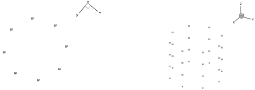
Figure 22: Generated cylindrical point cloud that is centered on the z-axis with a radius of 1 and a height of 2.
